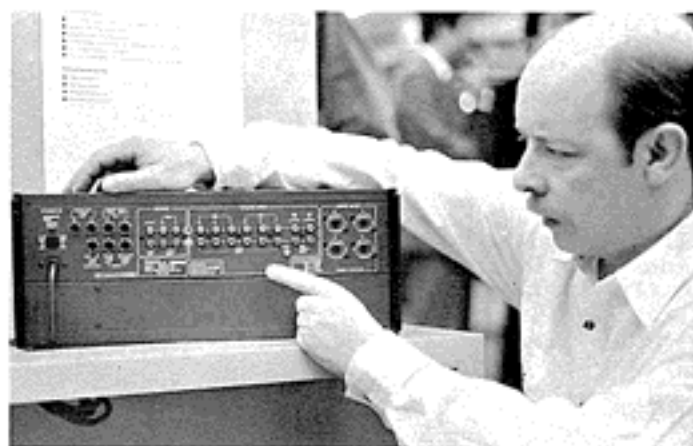
The WR-X01's simple control layout belies the number of inputs and outputs provided on the rear panel.
