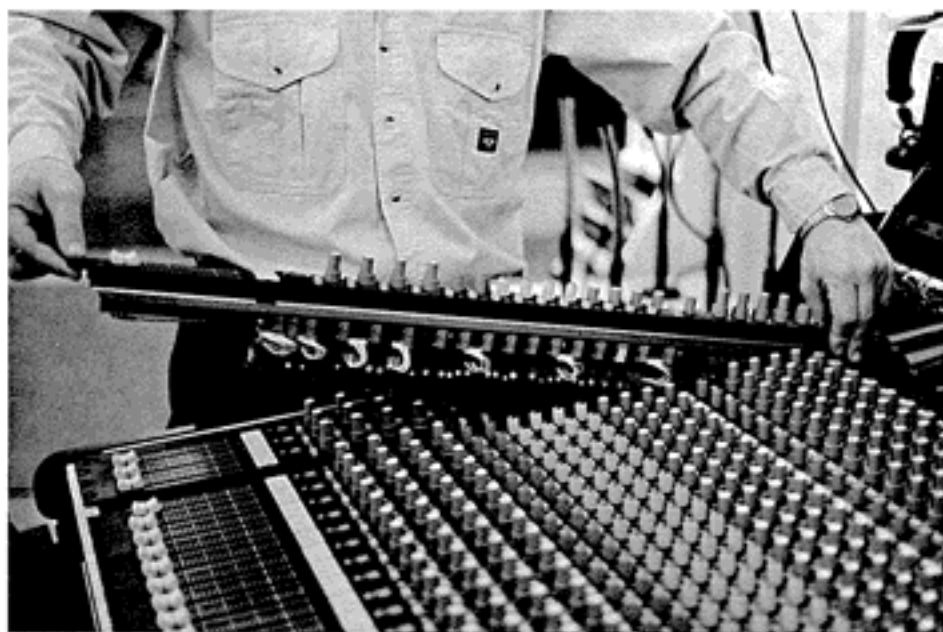
With the meter bridge removed, each module can be withdrawn, complete with their associated rear panel.
